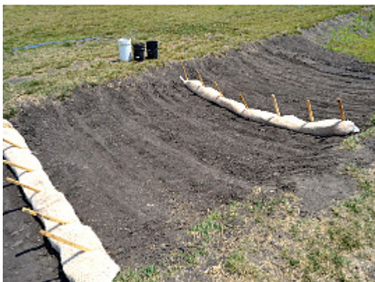
Figure S8. Sediment control log on an experimental plot (Bulnes Garcia 2013)
