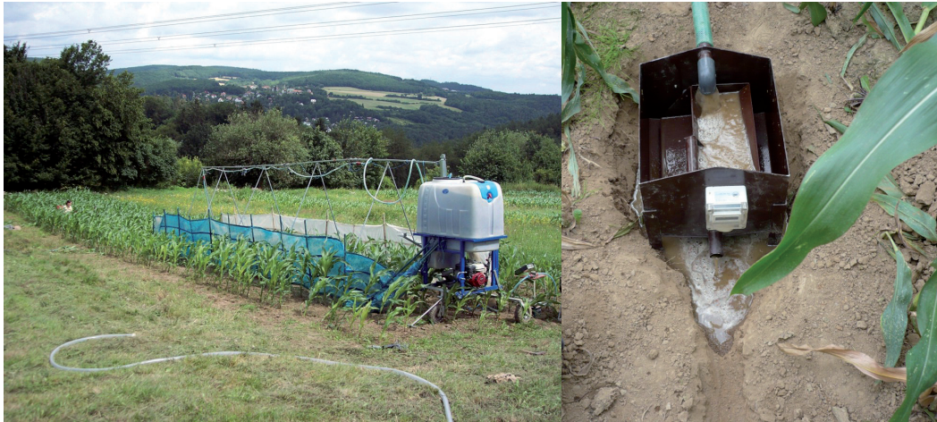
Figure 3. Left: rainfall simulator (RISWC Prague); right: discharge/sediment load measuring device (2009)
