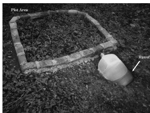
Figure 4. Established sample plot for estimating runoff during rainfall
