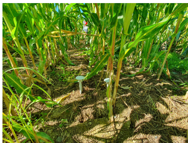
Figure 2. TMS-4 dataloggers during the maize vegetation period, strip-tilled plot
