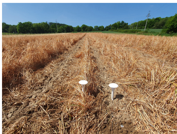
Figure 1. A pair of installed TMS-4 dataloggers prior to maize germination, strip-tilled plot
