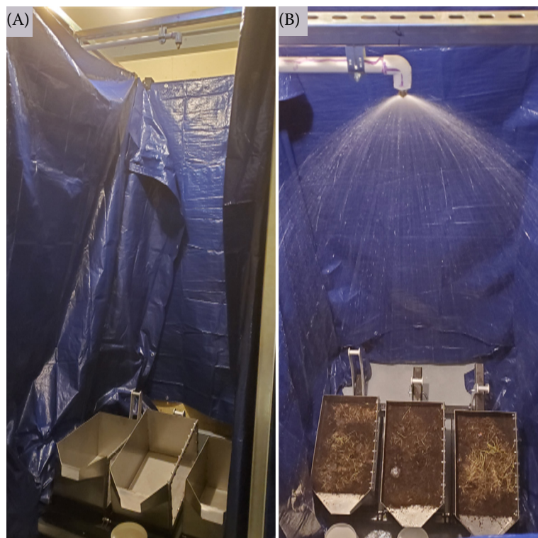
Figure 1. Images of the rainfall simulator (A) showing height of nozzle above microplots and the ability to independently tilt experimental microplots, and (B) an active rainfall simulation for the Control A group (undisturbed samples).
